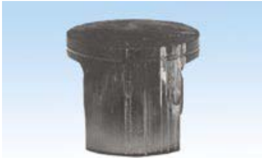
The piston ring (seen from the inlet side) is stuck in the groove and the dark discoloration under the piston ring is due to compression blow-by
