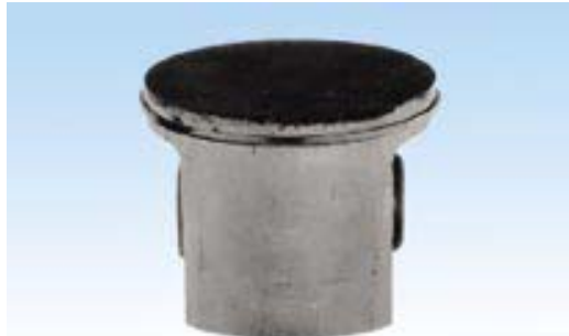
Small score marks and a matt, grey surface on the piston's inlet side caused by fine dust particles
