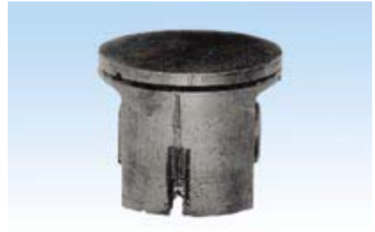
Extensive damage to the lower part of the piston's inlet side
