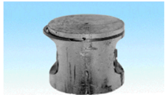
Irregular grooves on the piston's inlet side caused by a broken roller retainer
