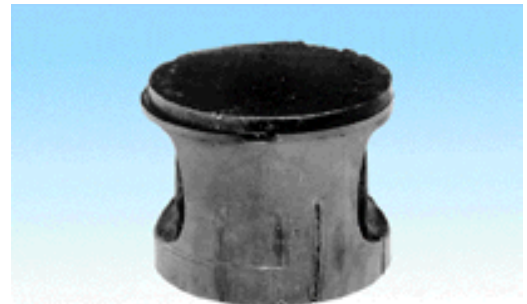
Deep, irregular grooves caused by a loose circlip is here shown here on the piston's inlet side
