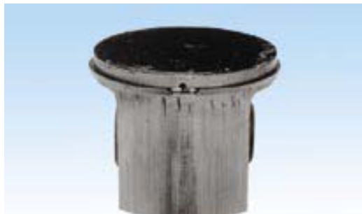
The piston scored and worn from the piston ring down on the inlet side
