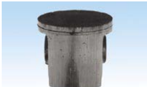
Particles of dust and dirt from carbon-like deposits on the top of the piston and in the piston ring groove
