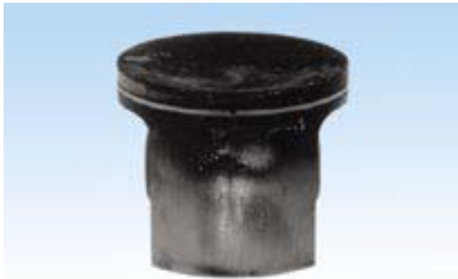
Medium to deep scores on the exhaust side. The piston ring is stuck in the groove. Dark discoloration under the piston ring due to compression blow-by
