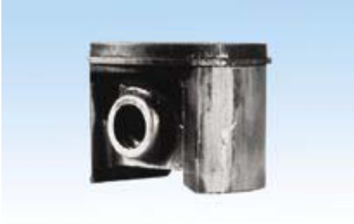
Small to medium scoring within the exhaust port area
