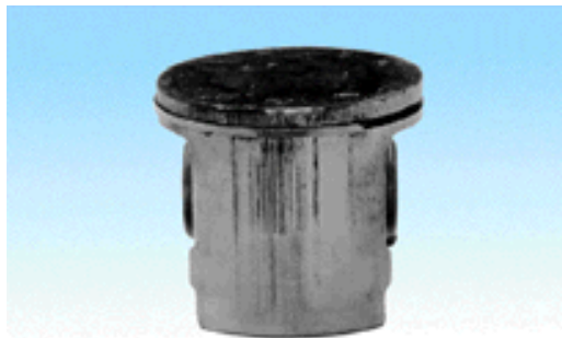
Exhaust side damaged by a broken piston ring. The piston ring parts damage the top section and cause score marks
