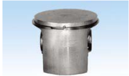
New piston from the inlet side
