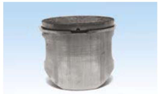
Piston from the inlet side with normal wear and normal discolouring
